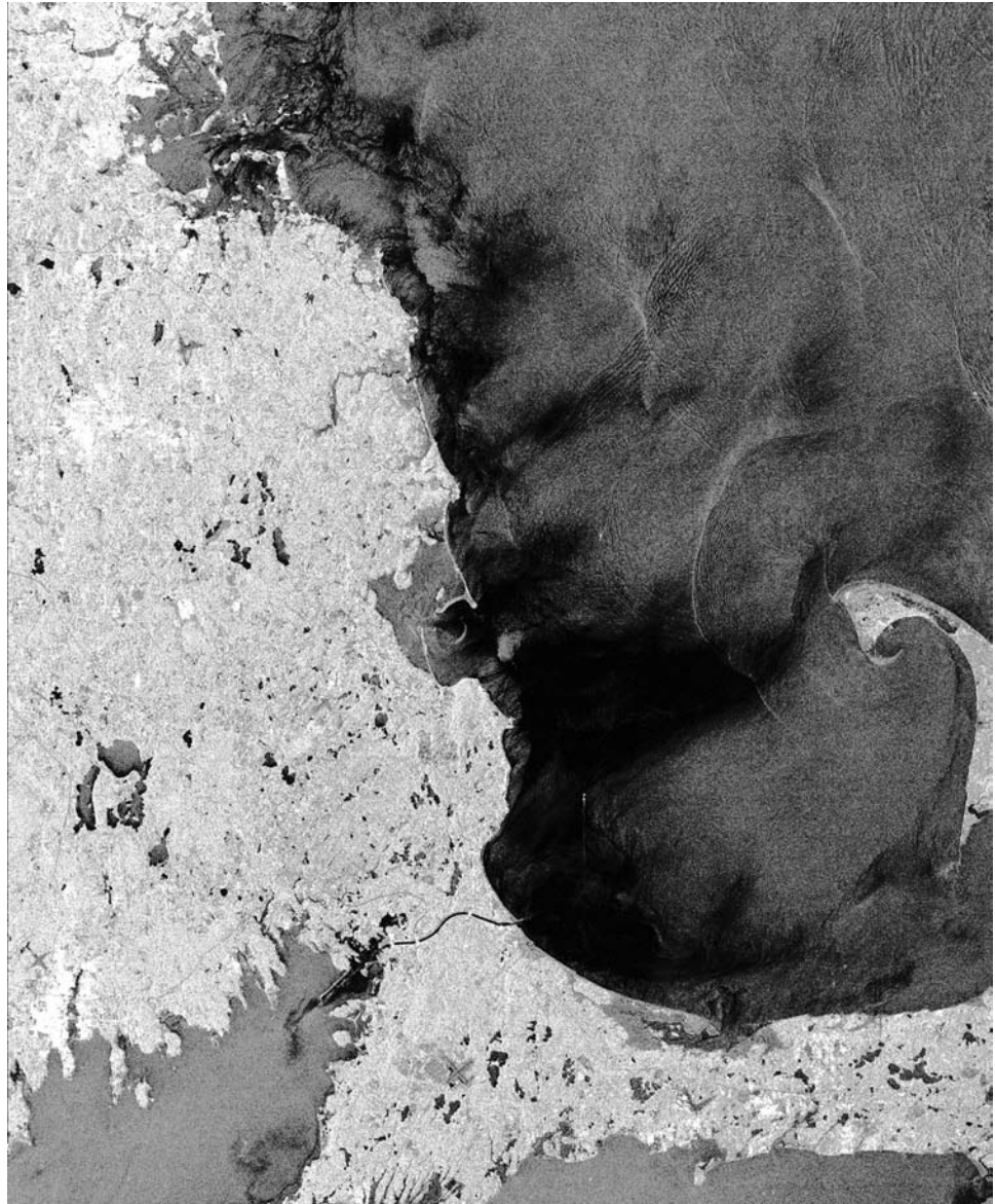
FIGURE 14. SYNTHETIC APERTURE RADAR (SAR) IMAGE OF INTERNAL WAVE EVENTS IN MASSACHUSETTS BAY ON AUGUST 7, 2003.
